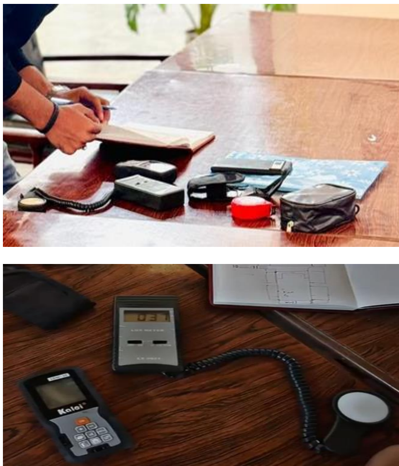
Figure 10. On-site documentation of the field survey, including observations of existing lighting conditions and the lux meter and measuring instruments used for illuminance measurements
