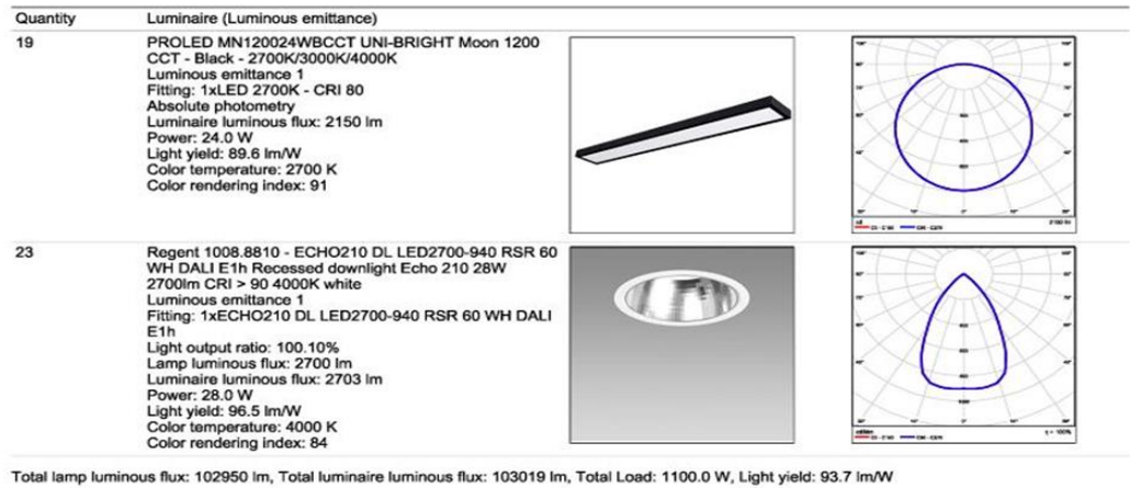
Figure 8. Types and specifications of luminaires used in the lighting simulation, reflecting the actual lighting setup of Montgomery Hall, Quaid-e-Azam Library, Lahore.
